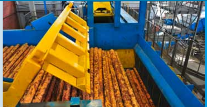
Loghandling and batch feeder for strander
